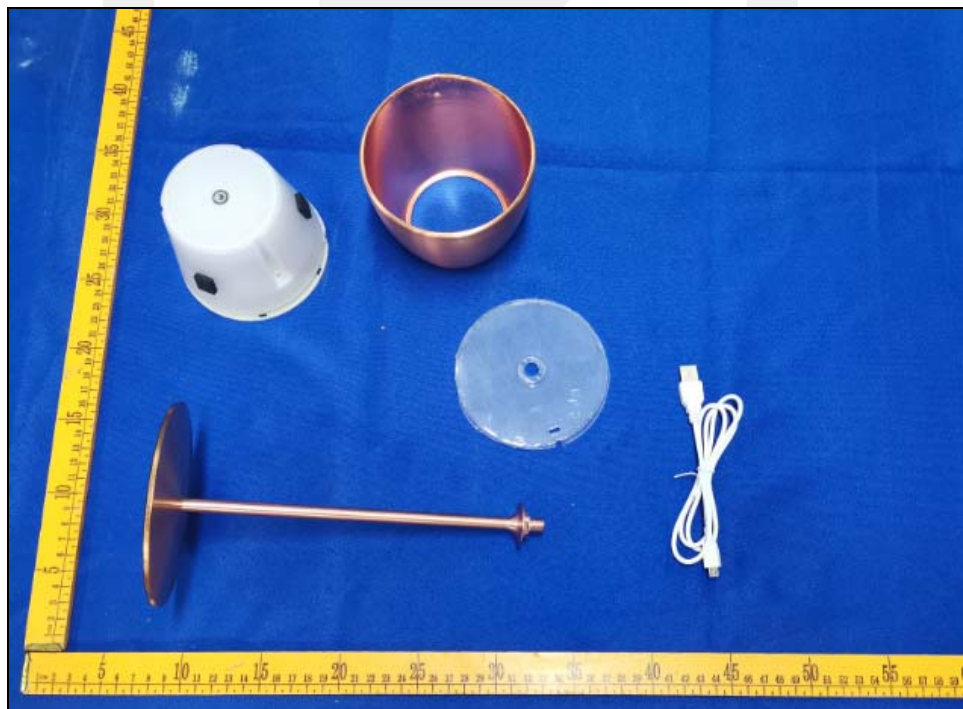
Figure 6: Separated view for model PBG-1230, Sally
